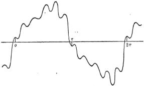
FIG. 44. Generator e.m.f. wave.
