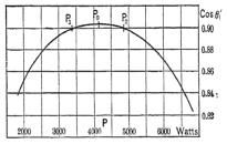
FIG. 53. Power-factor Maximum of Induction Motor.
