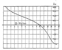
FIG. 58. First Differential Quotient of B, µ Curve
