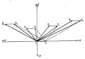
FIG. 18. Vector Diagram of Velocities of Steam in Turbine.
