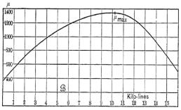
FIG. 52. Permeability Curve.
