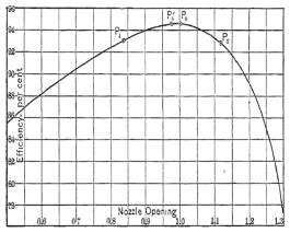
FIG. 54. Steam Turbine Nozzle Efficiency; Determination of Maximum.
