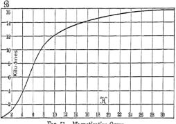
FIG. 51. Magnetization Curve.
