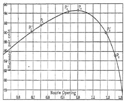
FIG. 55. Steam Turbine Nozzle Efficiency; Determination of Maximum.
