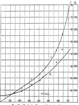
FIG. 59. Excitation Power of Induction Motor.
